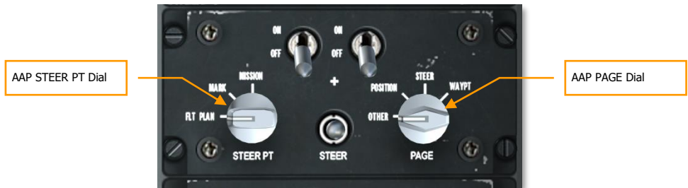
Figure 350. Auxiliary Avionics Panel (AAP)
