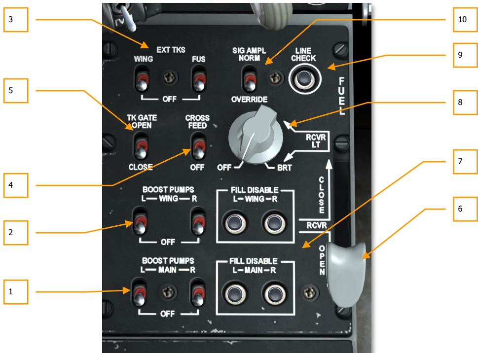
Figure 108. Fuel System Control Panel
