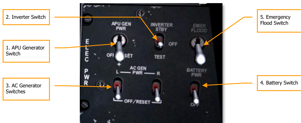
Figure 311. Electrical Power Control Panel
