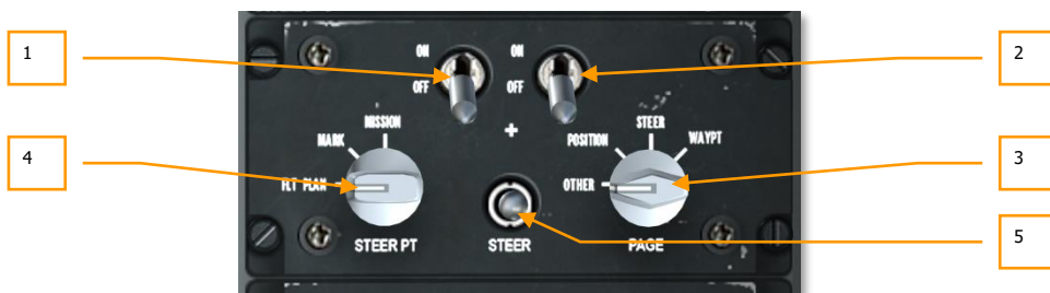
Figure 133. Auxiliary Avionics Panel (AAP)
