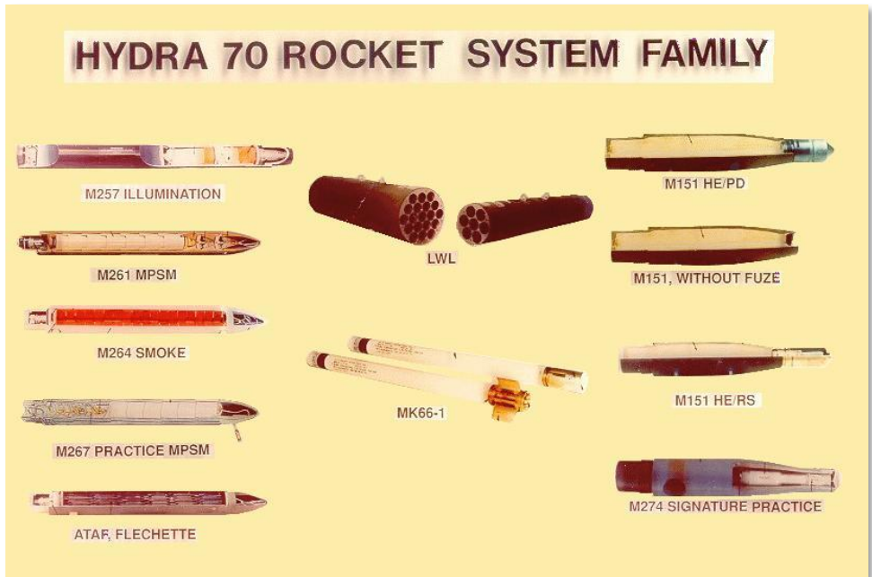
Figure 45. 2.75-inch FFAR Warhead Types
