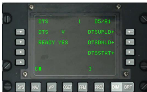
Figure 169. System / DTS Sub-Page
