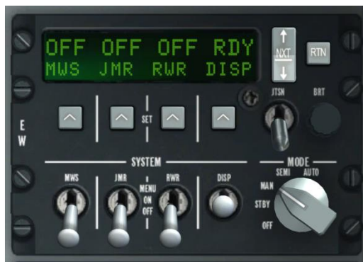
Figure 298. CMSP Dispenser ON
