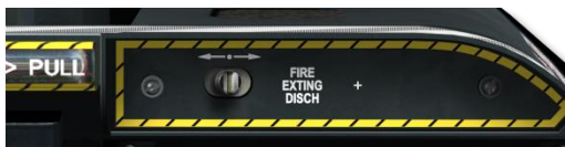
Figure 94. Fire Extinguisher Discharge
