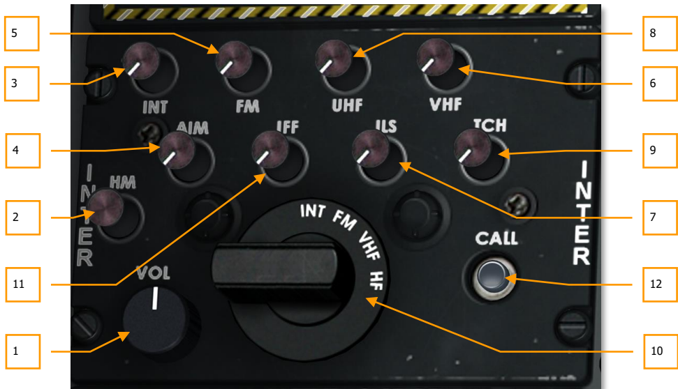
Figure 121. Intercom Control Panel
