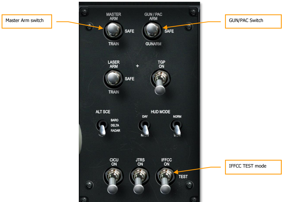
Figure 410. Armament HUD Control Panel
