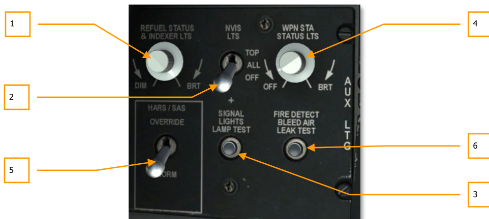
Figure 117. Auxiliary Lighting Control Panel
