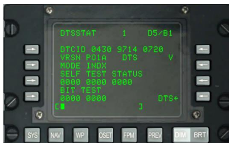
Figure 172. System / DTS Status Sub-Page
