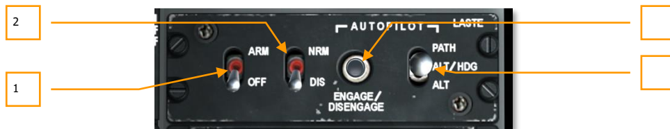
Figure 110. LASTE Control Panel
