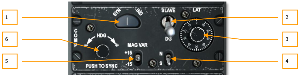
Figure 131. HARS Control Panel
