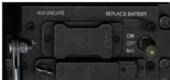
Figure 132. HMCS Control Panel
