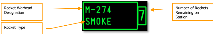
Figure 418. Rocket Loaded Station
