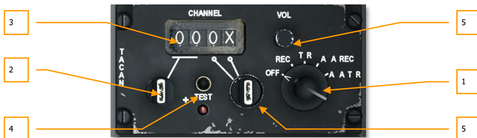
Figure 129. TACAN Control Panel
