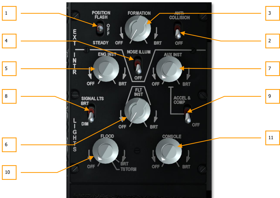
Figure 127. Light Control Panel
