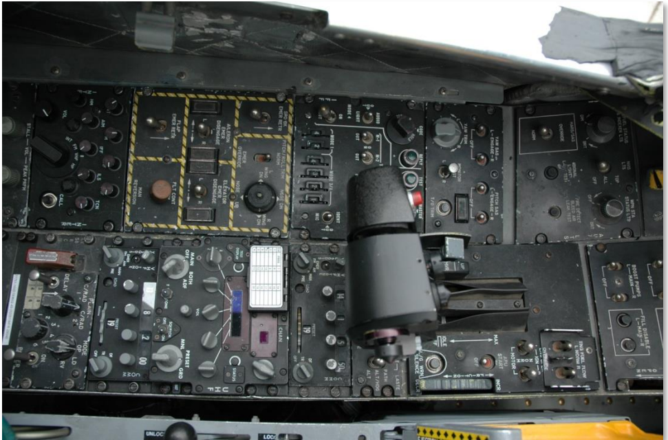
Figure 38. Left Console Showing VHF and UHF Radios
