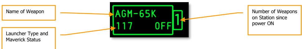
Figure 470. Maverick Station Box Loading, Power Off
