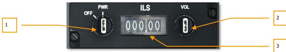
Figure 130. ILS Control Panel
