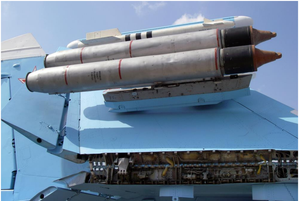
Figure 24: Heavy rockets S-25 on the double rack under wing
