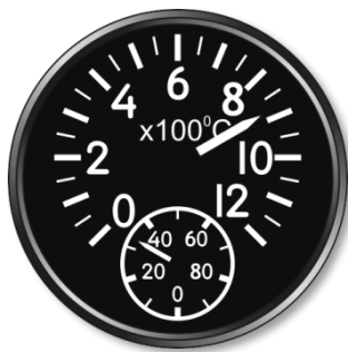
Figure 40: Interstage turbine temperature indicators
