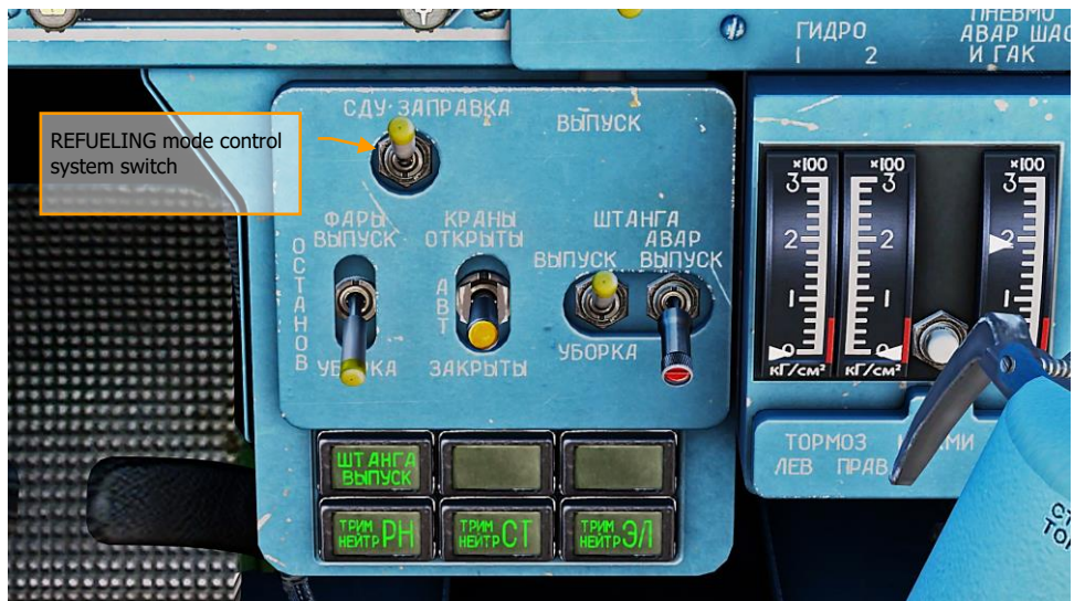
Figure 50: REFUELING mode control system switch
