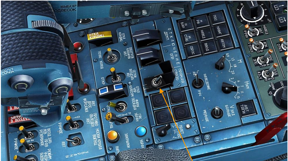
Figure 44: Direct control switch
