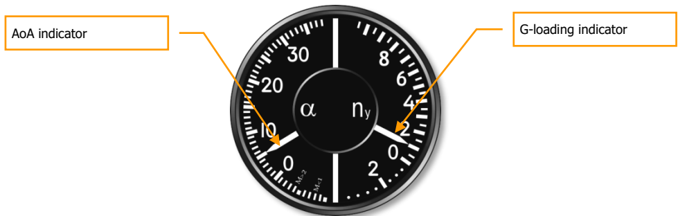
3-6: AoA indicator and Accelerometer
