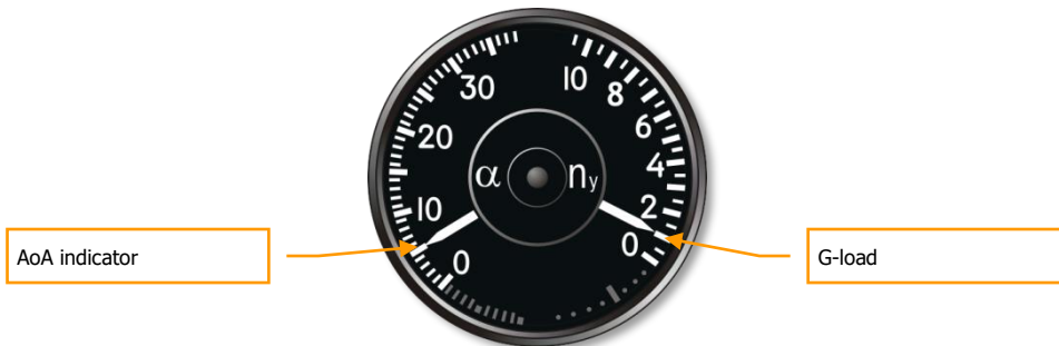
3-40: AOA Indicator and Accelerometer
