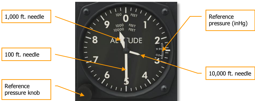
Figure 45: AN5760-2 Pressure Altimeter indicating 29,500 ft.
