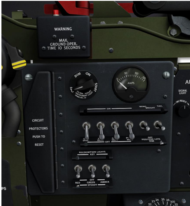
Figure 26: Electrical Control Panel
