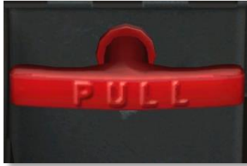
Figure 63: Landing Gear Fairing Door Emergency Release Handle
