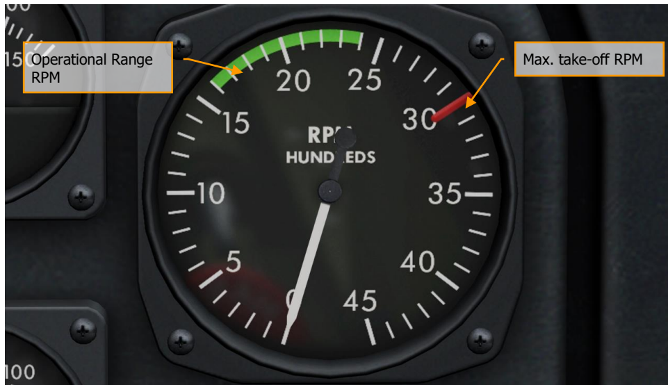
Figure 85: Max. take-off RPM 3000. Operating Range 1600...2400.
