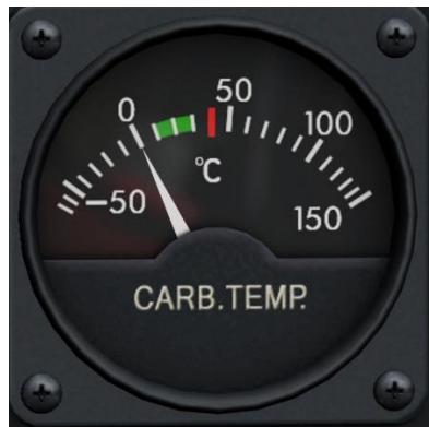
Figure 49: Carburetor Air Temperature Indicator
