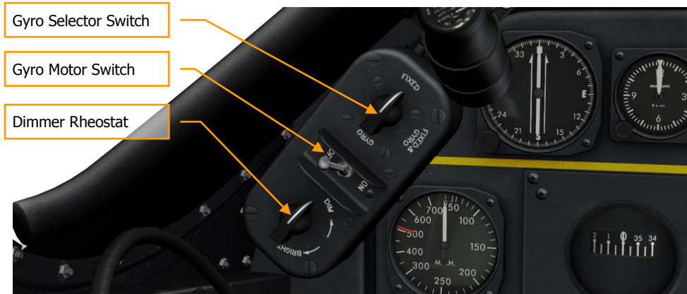
Figure 38: K-14 gunsight selector-dimmer panel
