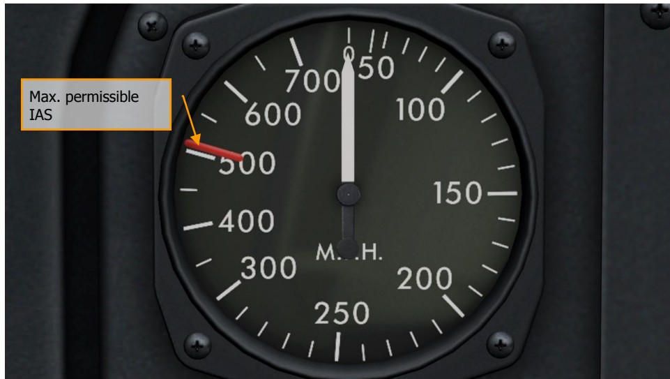
Figure 86: Max. permissible IAS 505 mph (808 km/h, 440 knots)
