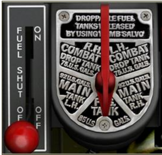
Figure 19: Fuel Selector Valve
