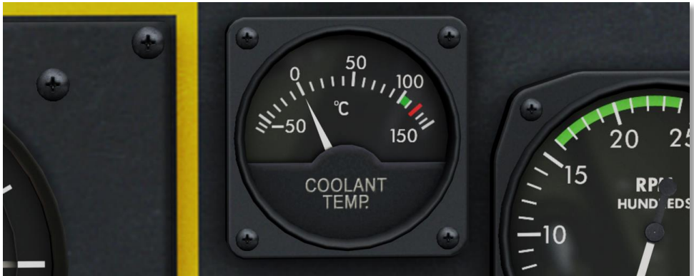
Figure 87: Max. coolant temperature 121°C (250°F), operating range 100...110°C (212...230°F)
