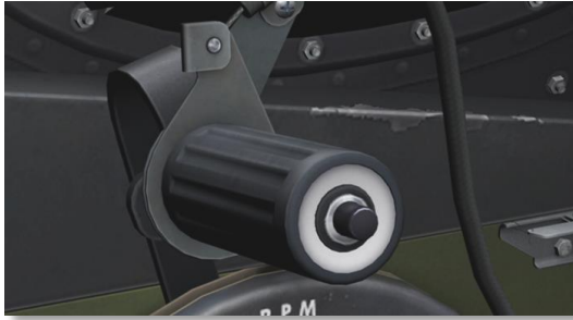
Figure 95: Throttle Control handle with twist grip
