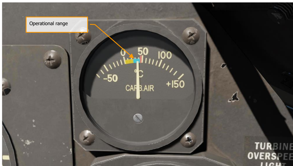
Figure 89. Carburetor air temperature operational range 0 - 40°C, max. temperature +50°C
