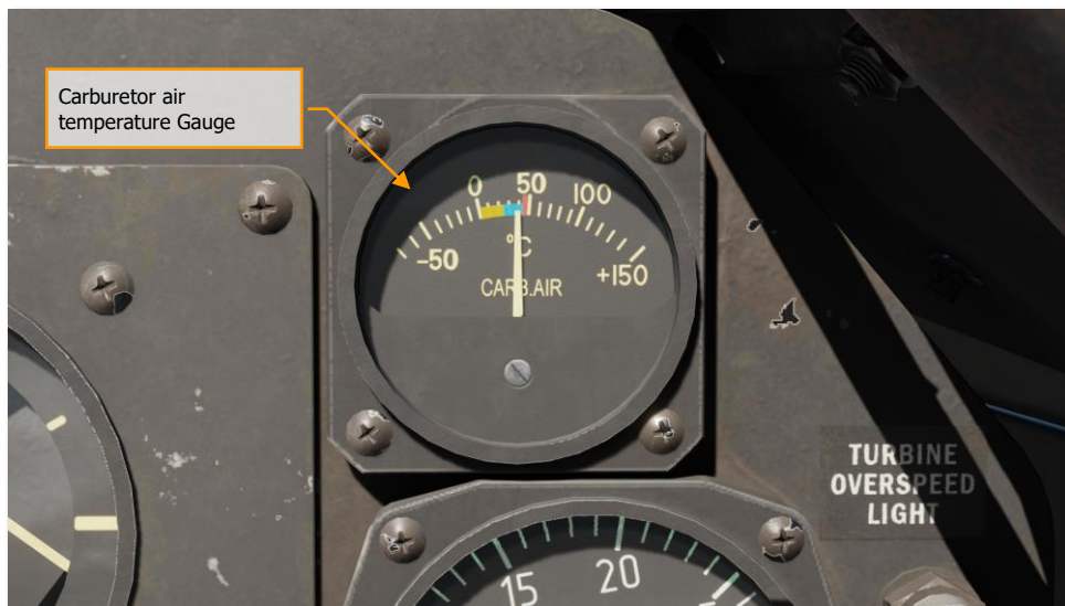
Figure 53. Carburetor air temperature Gauge
