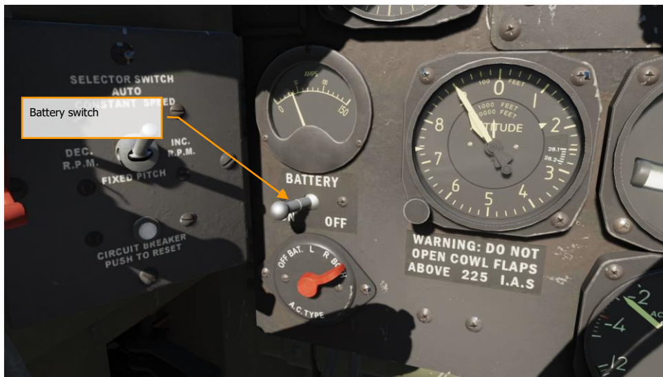
Figure 68. Battery control switch
