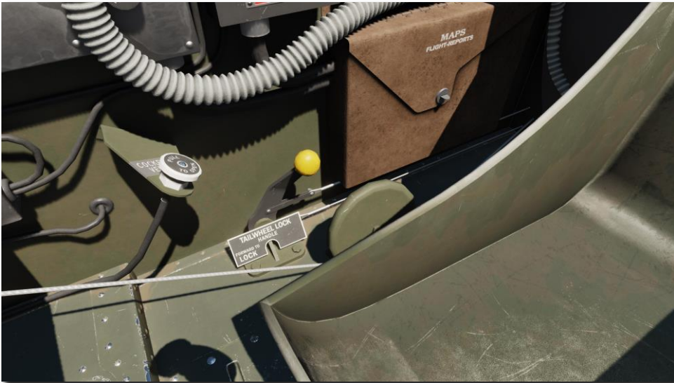
Figure 76. Tail wheel lock control handle
