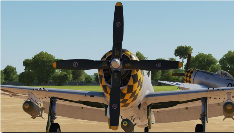
Figure 20. Curtiss Electrics 4-bladed constant speed propeller
