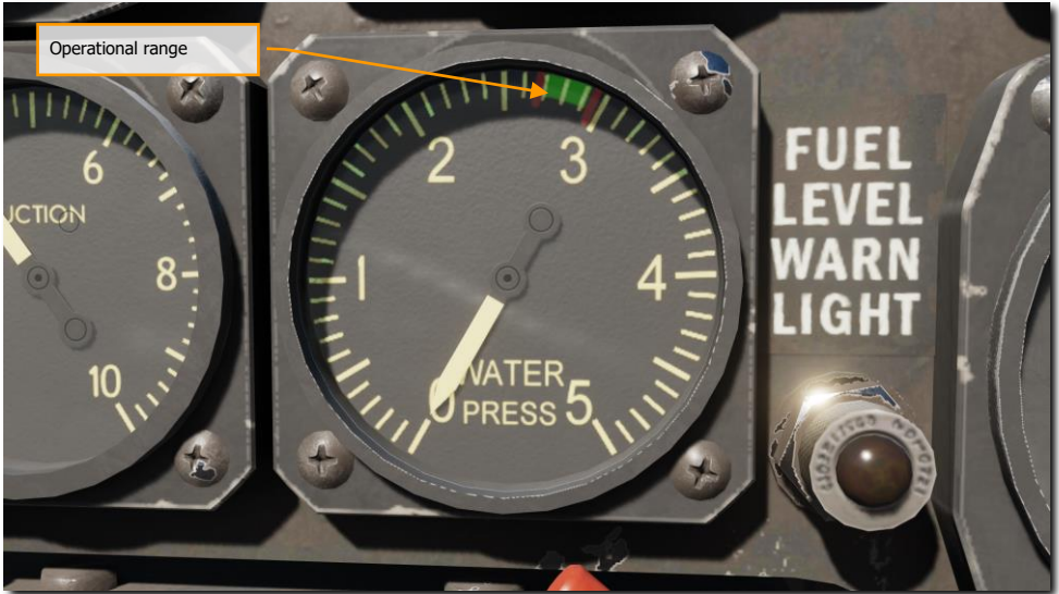
Figure 91. Operational water pressure range is 25-27PSI
