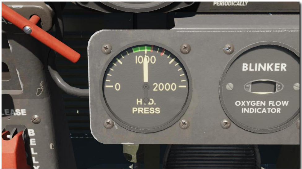
Figure 63. Hydraulic pressure gauge
