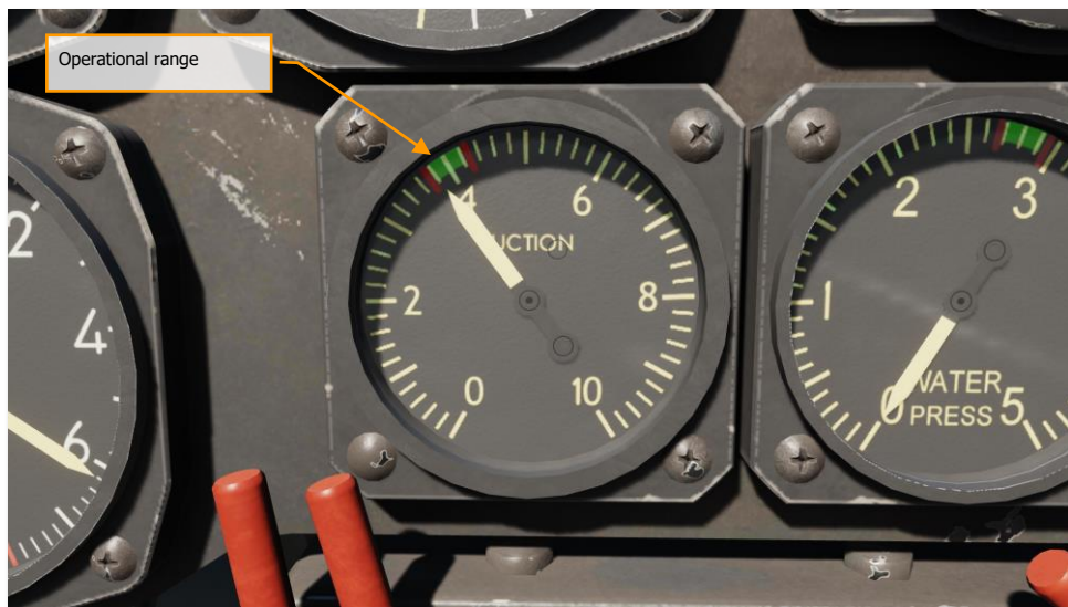
Figure 90. Operational vacuum range— 4.00 in. Hg.
