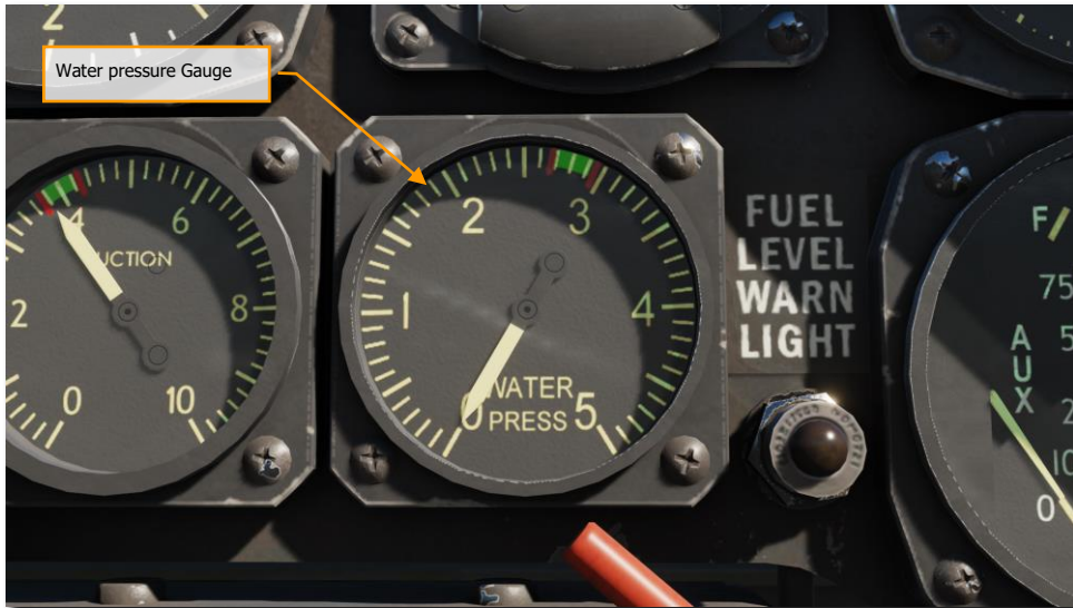
Figure 61. Water pressure Gauge
