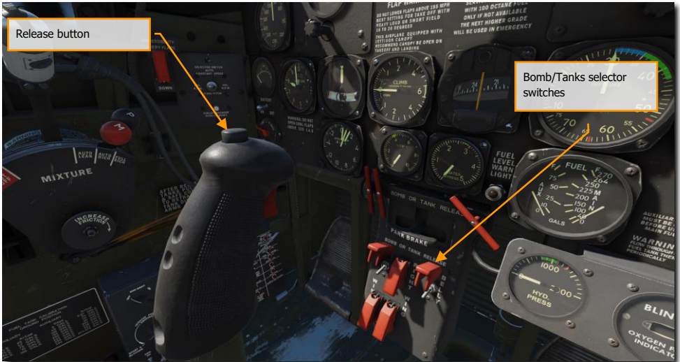
Figure 93. Bomb/Tank selector switches
