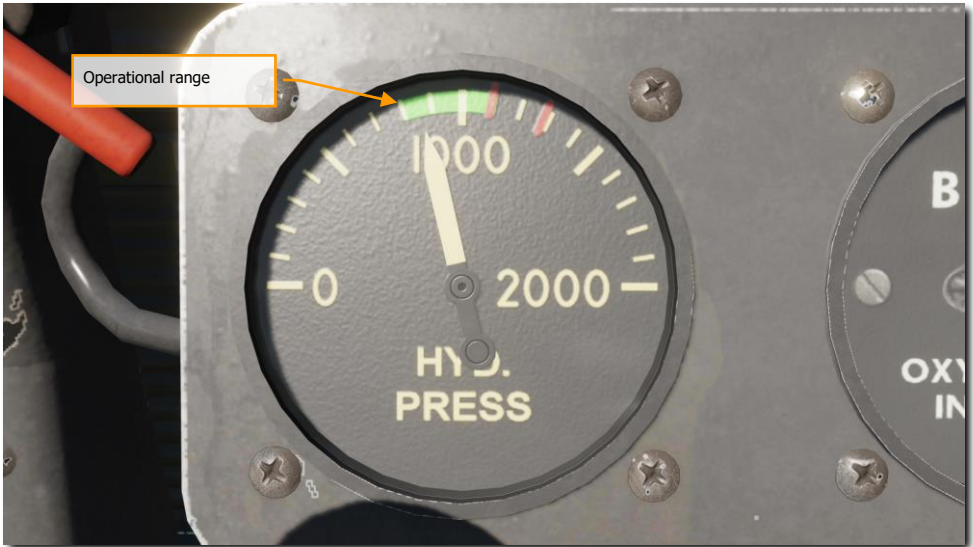
Figure 92. Operational hydraulic pressure range is 800-1100PSI. Maximum hydraulic pressure - 1300PSI
