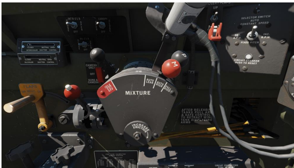
Figure 81. Mixture control lever (M) and propeller control lever (P)
