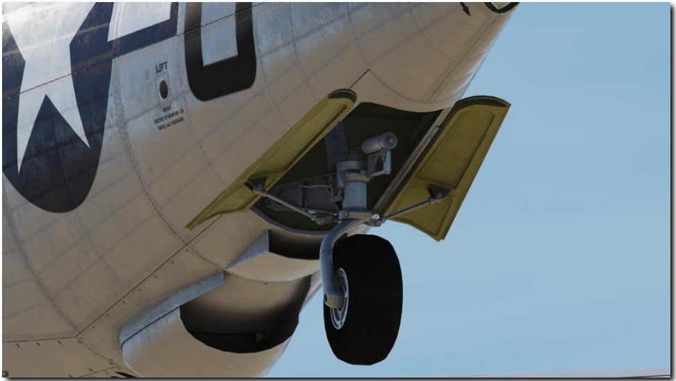
Figure 16. Hydraulically retractable tailwheel
